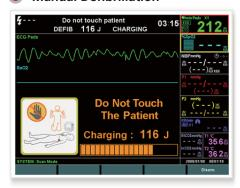
Biphasic Manual Defibrillation with maximum Energy level of 360 J. With Synchronous Cardioversion.
