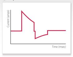
Most effective Biphasic Truncated Exponential Waveform with impedence compensation. (25 to 175 Ohm)
