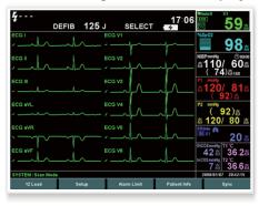
Full range of monitoring options available, including 3/5/12 Lead ECG (Glasgow University), Nellcor SpO2, Omron NIBP, IBP, Temp and Respironics EtCO2.
